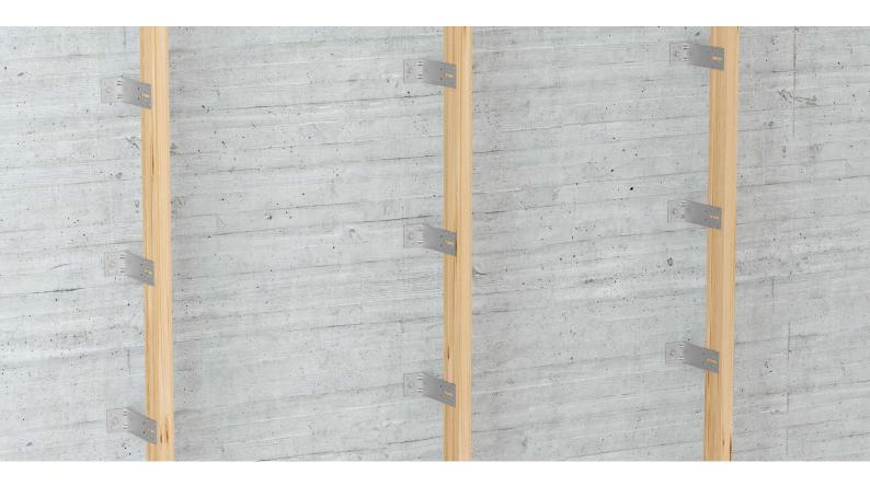
Console angles are used for façades placed in front of timber sub-structures. The necessary bracket size must be chosen in relation to the insulation thickness. The short leg is for fastening to the façade. The long leg is for fixing the frame left (substructure) with screws or nails (under compliance with the necessary minimum edge spacing).
