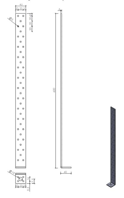
Figure B. 11 Dimensions of type HSB 600x40x40x4,0
