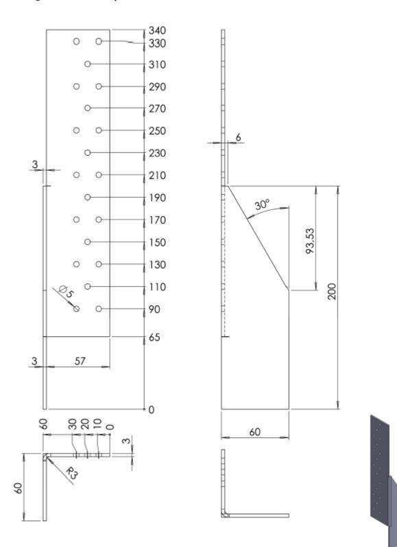
Figure B.54 GH-HT2 SB Zuglasche li 340x60/60x3,0
