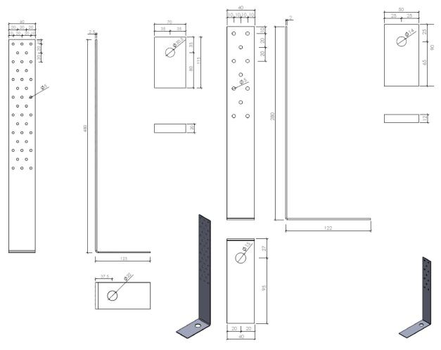
Figure B. 16 Dimensions of type 480x123x60x2,5
