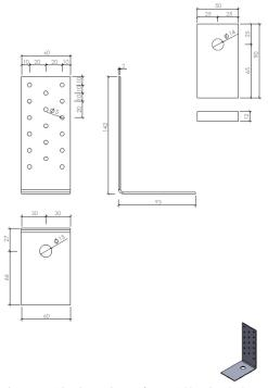
Figure B. 18 Dimensions of type 142x93x60x2
