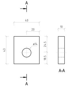
Figure B. 26 Dimensions of washer for type HB and HSB
