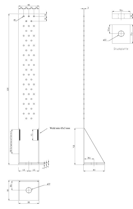
Figure B. 32 Dimensions of type GH HT34 80/620 (drawing with washer 77x70x20)
