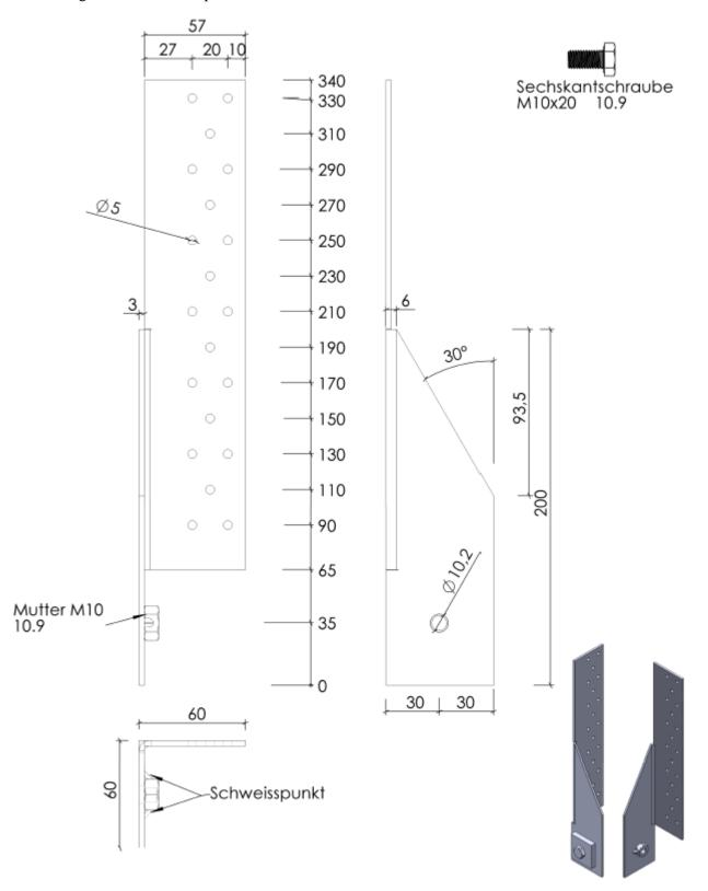
Figure B.48 GH-HT2 SM Zuglasche Li 340x60/60x3,0mm
