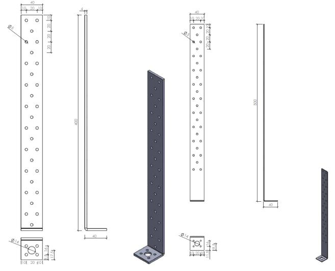
Figure B. 7 Dimensions of type HSB 400x40x40x4,0
