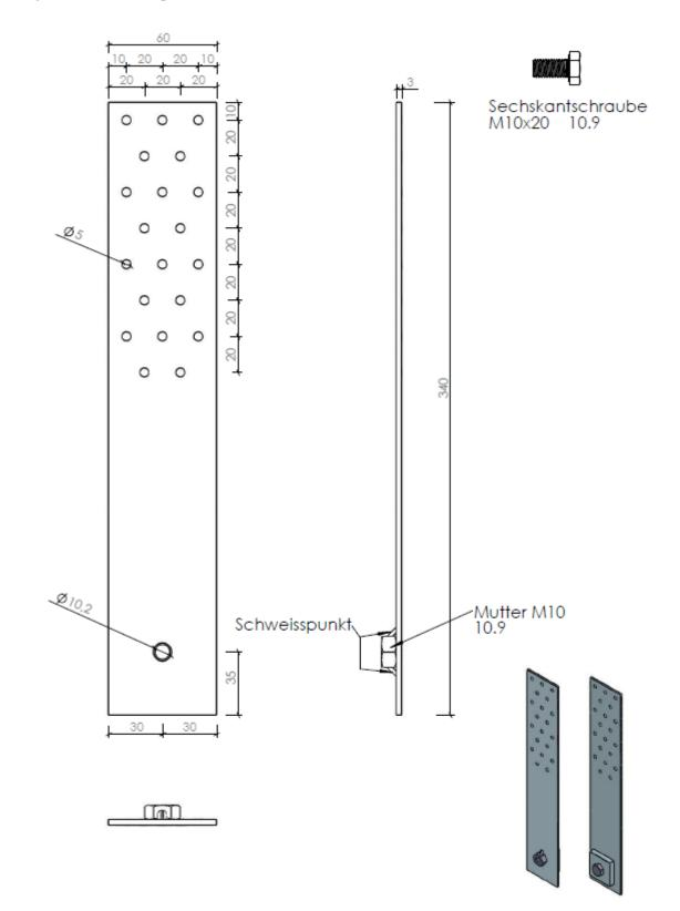
Figure B.47 GH-HT2 SM Zuglasche G 340x60x3,0mm
