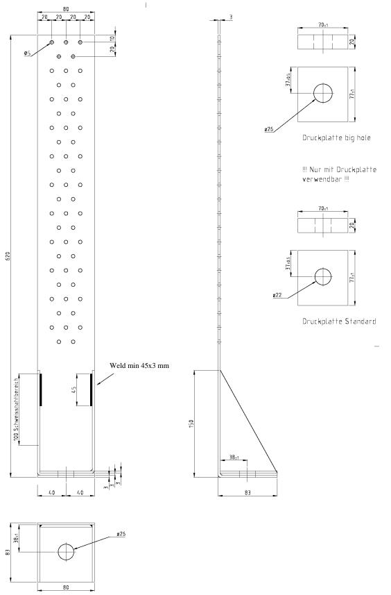
Figure B. 34 Dimensions of type GH HT34 80/620 Big hole (with washer 77x70x20xØ22 or 77x70x20xØ26 )
