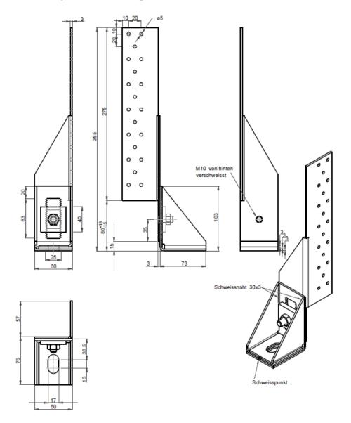
Figure B.44 HT2-RV-340-Stegwinkel-Z-225
