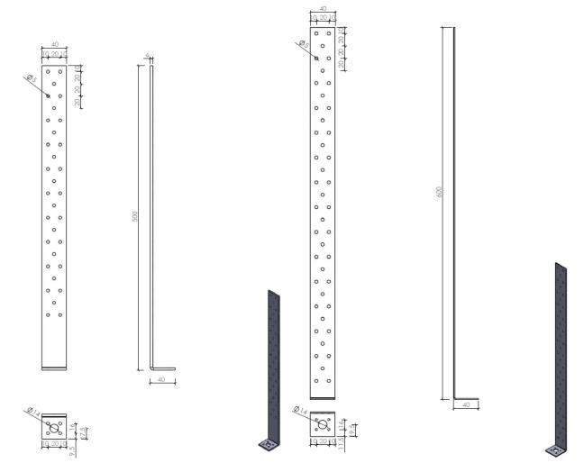
Figure B. 9 Dimensions of type HSB 500x40x40x4,0
