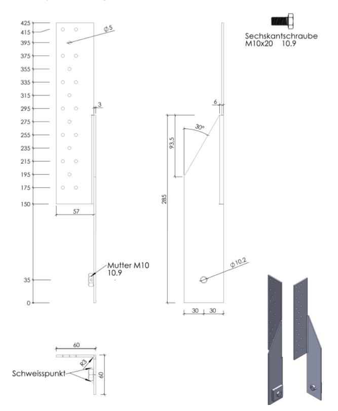
Figure B.51 GH-HT2 SM Zuglasche re 425x60/60x3,0mm
