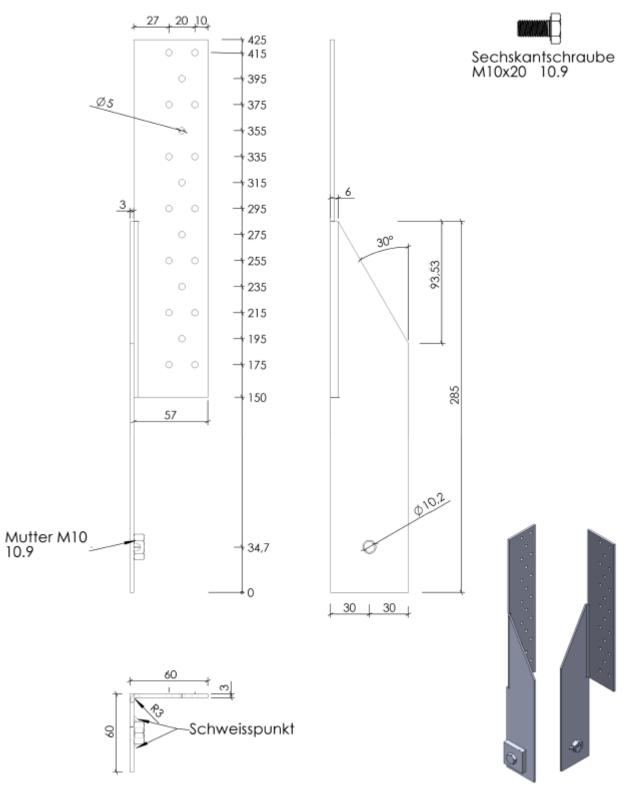
Figure B.50 GH-HT2 SM Zuglasche li 425x60/60x3,0mm
