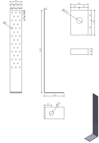
Figure B. 15 Dimensions of type 420x102x60x2,0
