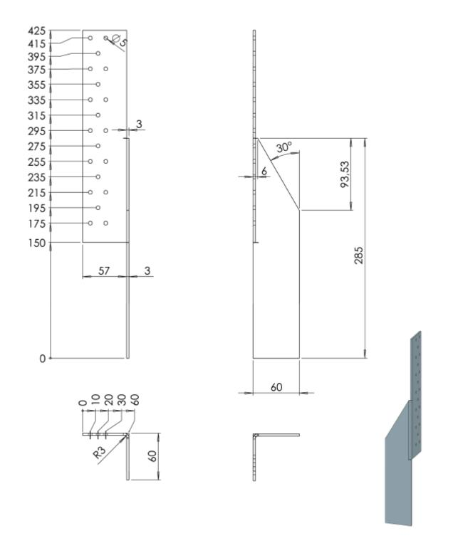
Figure B.59 GH-HT2 SB Zuglasche re 425x60/60x3,0
