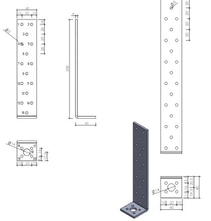
Figure B. 2 Dimensions of type HSB 200x40x40x2,0
