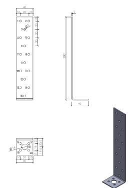
Figure B. 1 Dimensions of type HB 155x50x40x3,0
