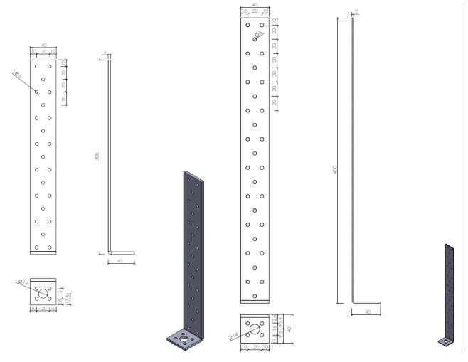
Figure B. 5 Dimensions of type HSB 300x40x40x4,0
