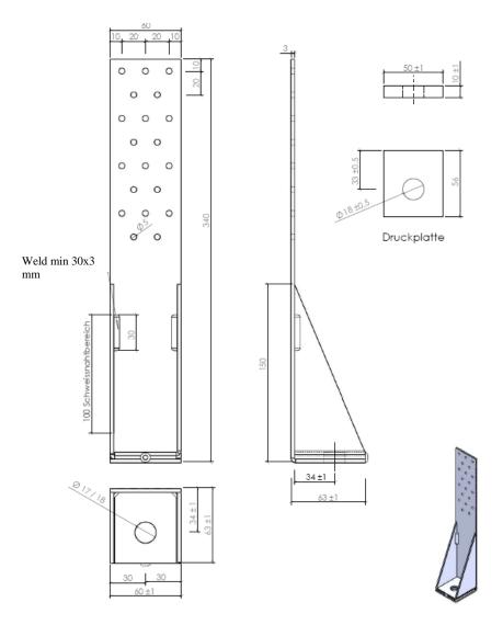
Figure B. 27 Dimensions of type GH HT16 60/340 (drawing with washer 56x50x10)
