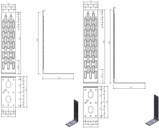
Figure B. 20 Dimensions of Top Vario 240x120x55x2,0
