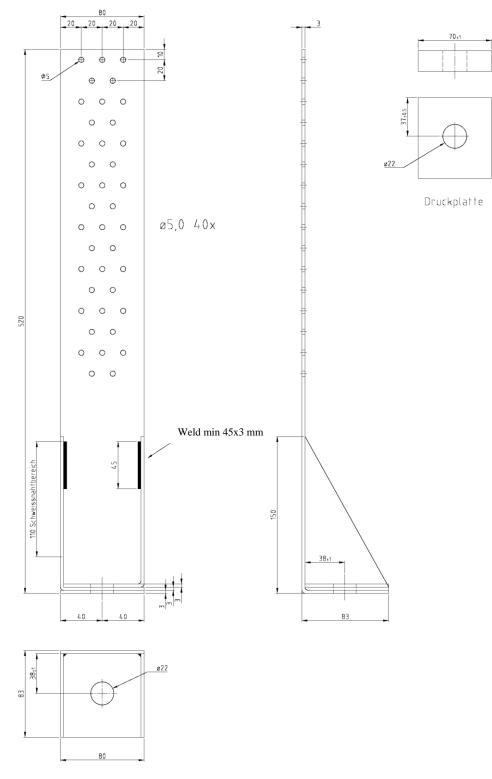
Figure B. 31 Dimensions of type GH HT32 80/520 (drawing with washer 77x70x20)
