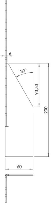
Figure B.55 GH-HT2 SB Zuglasche re 340x60/60x3,0
