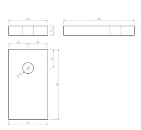
Figure B. 24 Dimensions of washer for hold-down 520x222x60x2,5
