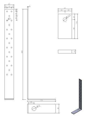
Figure B. 13 Dimensions of type 400x123x40x3,0
