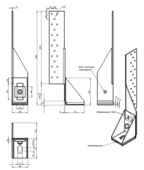
Figure B.42 HT2-LV-340-Stegwinkel-Z-220
