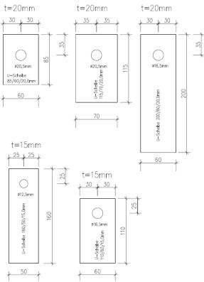
Figure B. 23 Dimensions of washers for hold-downs
