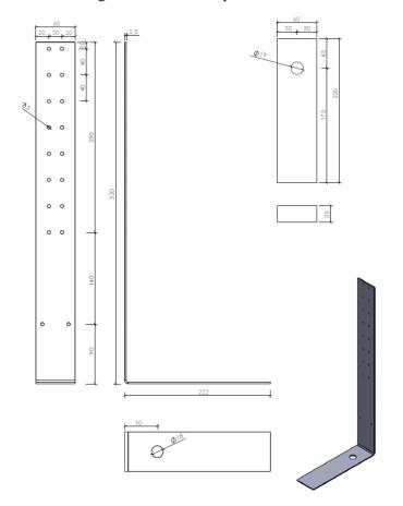
Figure B. 19 Dimensions of type 520x222x60x2,5
