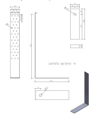
Figure B. 14 Dimensions of type 420x222x60x2,0
