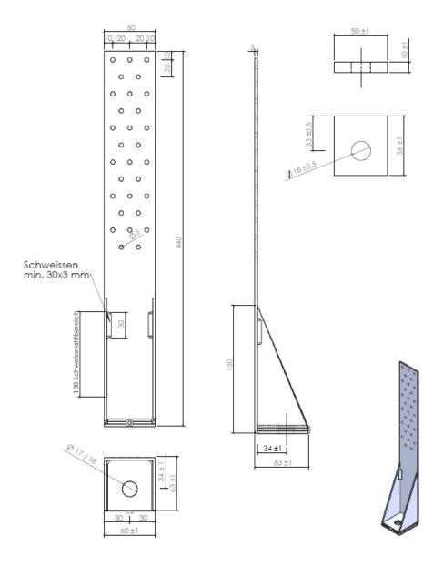
Figure B. 28 Dimensions of type GH HT22 60/440 (drawing with washer 56x50x10)
