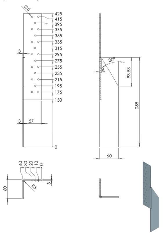
Figure B.58 GH-HT2 SB Zuglasche li 425x60/60x3,0
