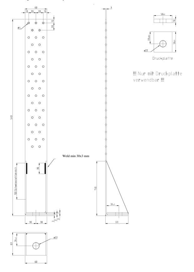
Figure B. 33 Dimensions of type GH HT28 60/540 Big Hole (with washer 56x50x10)
