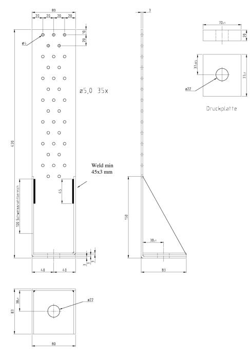
Figure B. 30 Dimensions of type GH HT30 80/420 (drawing with washer 77x70x20)
