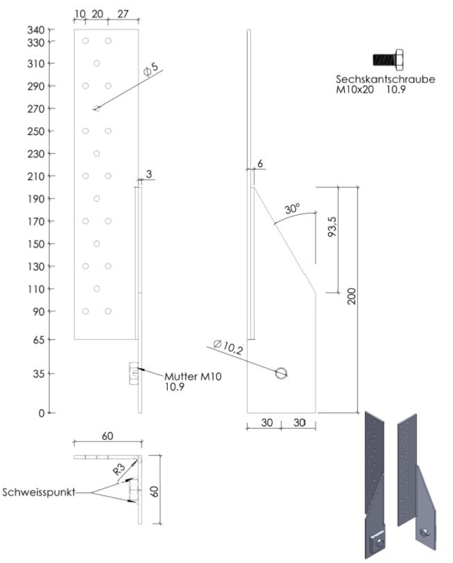
Figure B.49 GH-HT2 SM Zuglasche re 340x60/60x3,0mm
