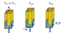
$$\label{eq:F1} \begin{split} F_{1,c} & - \text{compressive force (downwards) perpendicular to the baseplate} \\ F_{1,t} & - \text{tensile force (upwards) perpendicular to the baseplate} \\ F_{2/3} & - \text{load perpendicular to fasteners in the fin, dowel, ties} \\ F_{4/5} & - \text{load parallel to fasteners in the fin, dowel, ties} \end{split}$$
