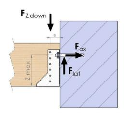
The resistances shown result for the fixing with a pair of dowels, bolts or concrete anchors. If the fixing is made with several dowel, bolt or concrete anchor pairs, the resistance of the joist hanger and the loading of each dowel, bolt or concrete anchor can be converted as follows:
