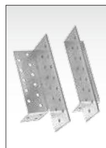
GH truss clips, 2-piece, are suitable for fixing rafters on joists. Removes the need for time-consuming offset and the inclined stud or clamping bolts. GH truss clips, 2-piece, are used for a timber width from approx. 80 mm.
