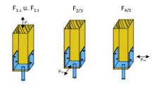
$F_{1,c}$  - compressive force (downwards) perpendicular to the baseplate  $F_{1,t}$  - tensile force (upwards) perpendicular to the baseplate  ${\rm F}_{\rm 2/3}$  - load perpendicular to fasteners in the fin, dowel, ties  $\mathsf{F}_{4/5}$  - load parallel to fasteners in the fin, dowel, ties
