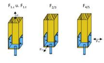
$F_{1,c}$  - compressive force (downwards) perpendicular to the baseplate  $F_{1,t}$  - tensile force (upwards) perpendicular to the baseplate  $F_{2/3}$  - load perpendicular to fasteners in the fin, dowel, ties  $F_{4/5}$  - load parallel to fasteners in the fin, dowel, ties
